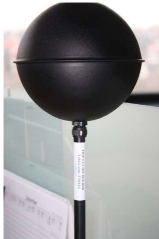
TESTO 6055/0600 9999 radiation temperature measurement equipment
